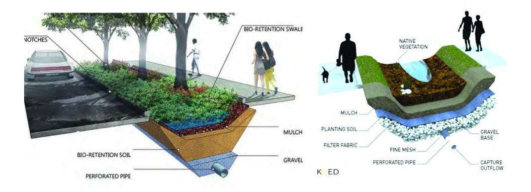
Typical design of a bioswale of city street
