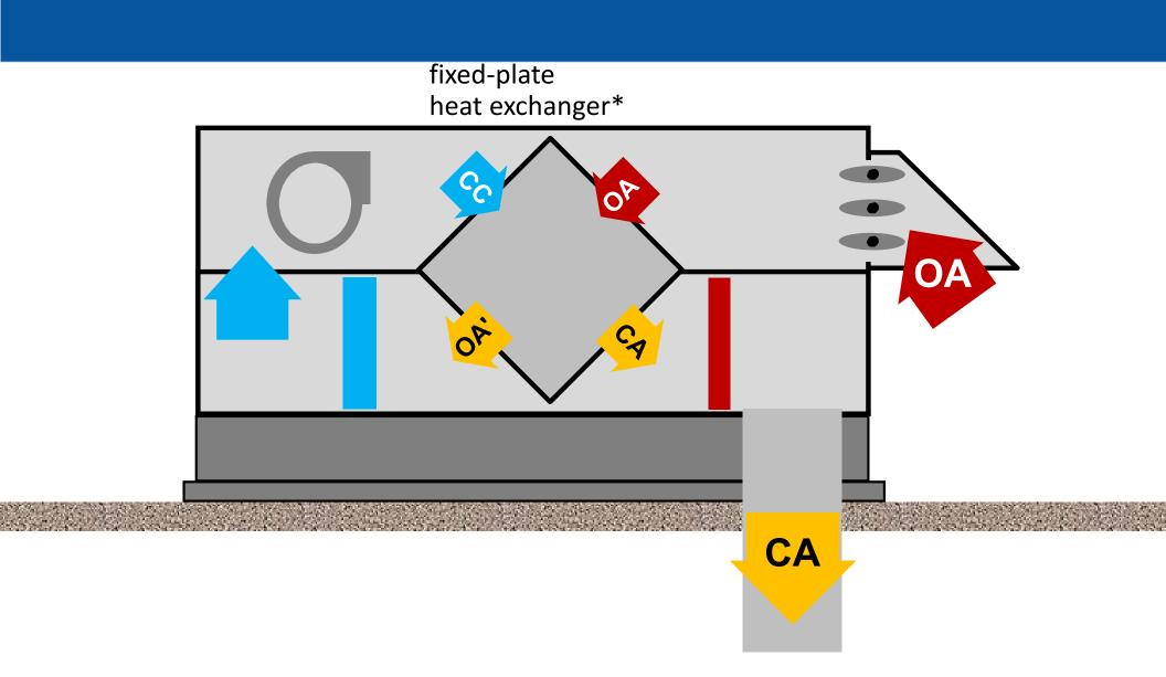
\* could also be a heat pipe, coil loop, or sensible heat wheel
